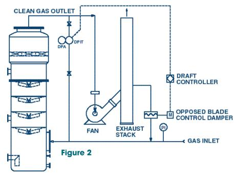
The RotaBed Plus<sup>™</sup> using a special precleaning section is able to remove TRS compounds with greater removal efficiency than wet dynamic and venturi scrubbers.
